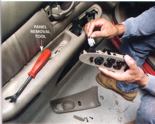
1 Pry out the switch panel and disconnect the electrical connectors. Then remove the door trim panel.
