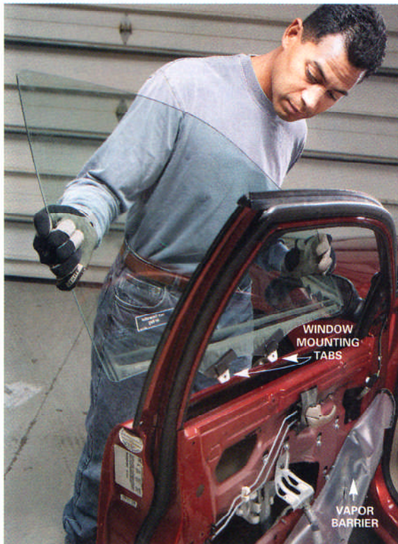
3 Remove the glass-to-regulator bolts (if needed, cut the mechanical cables to raise or lower the glass). Tilt the window up and out and set it in a safe place.
