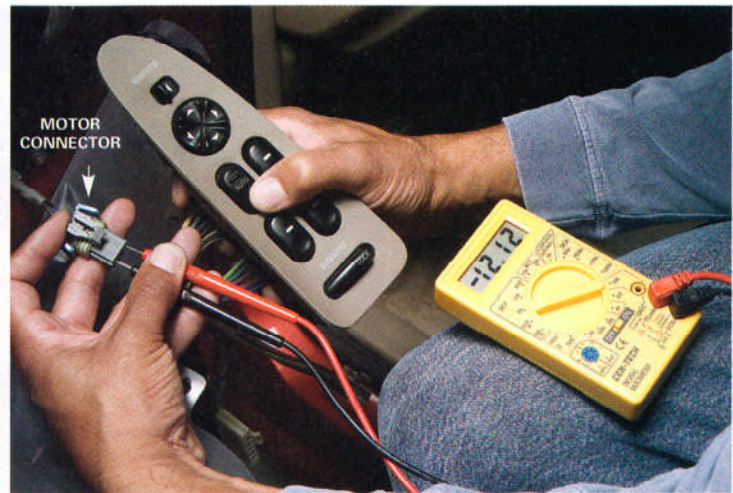
2 Reconnect the switch panel and attach the voltmeter test leads to the motor connector. Then toggle the window switch. If the switch is good, replace the regulator.
